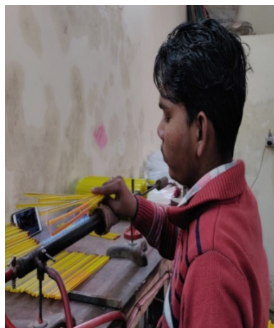
Figure 20. Making of Mercury-containing Thermometers in Ambala
