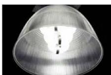
Induction lamps: Also called "electrodeless", they tend to have low mercury per lumen-hour and be very long-lasting (up to 100,000 hours or 11.4 years of continuous operation). They are generally used for high-bay applications such as warehouses or other places where it is difficult to change lamps (e.g., jails), but they may have high initial cost.
