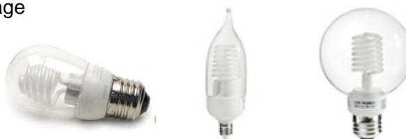
These lamps are typically long-lasting (15,000-25,000 hours) and dimmable and have low mercury (some 1 mg). They are generally used for low-watt, small-size applications such as bathroom vanities, marquees, sconces and chandeliers. Some CC CFLs are less efficient than standard CFLs (40 LPW vs 60 LPW) but all are more efficient than incandescents.
