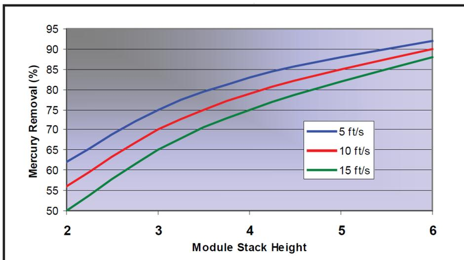
Figure 3: Stacked Modules Design for Desired Removal Efficiency
