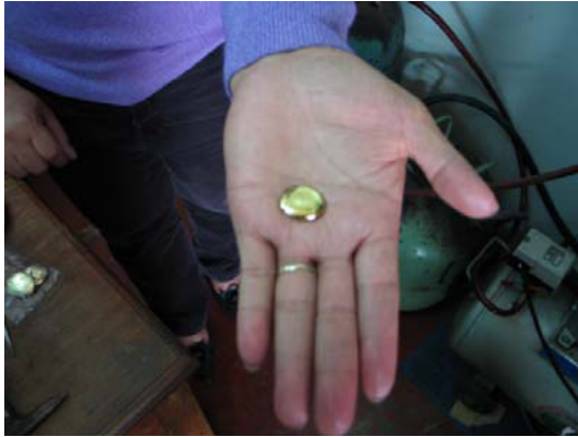
A pure gold pellet produced without use of mercury
