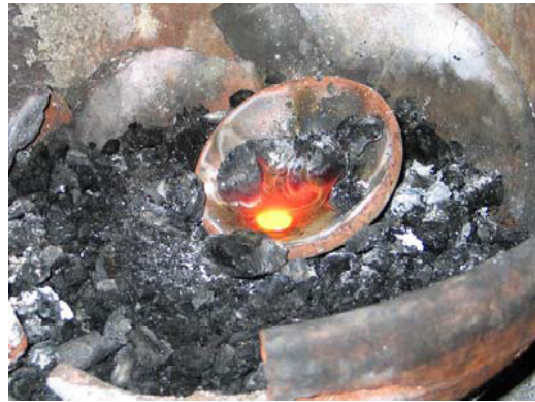
The shining gold pellet in red glowing molten borax
