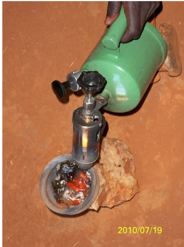
Melting of the ore by using kerosene stove which takes longer time
