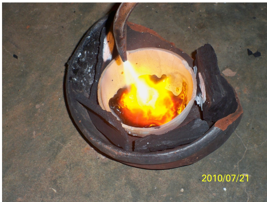
Melting concentrate of ore with Borax by using acetylene gas burner which takes shorter time
