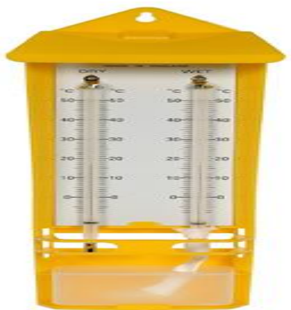
Figure 10: Showing a wet and dry bulb hygrometer for indoor or outdoor use with mercury filling.
