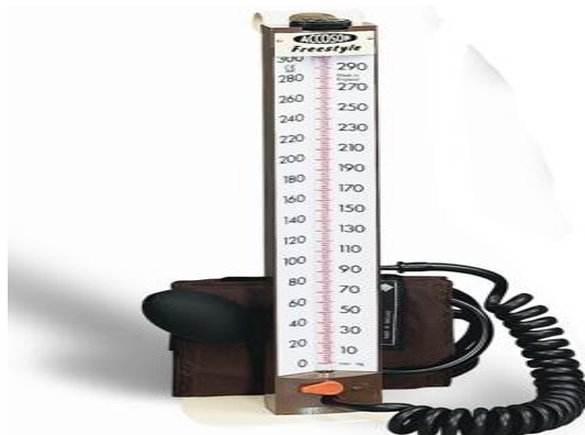
Figure 8: An example of a Freestyle Mercury Sphygmomanometer available
