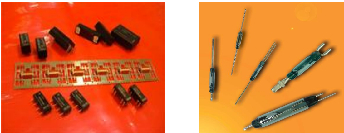
Figure 15: Mercury Wetted Relays and Mercury wetted reed switches also available in Nigeria
