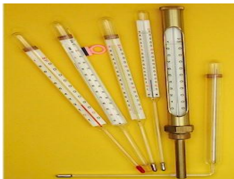
Figure 4: Shows some examples of mercury-containing thermometers
