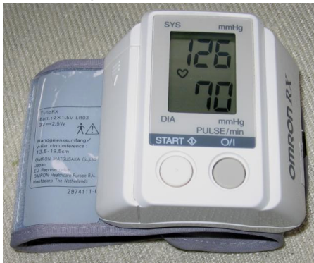
Figure 5 – The Omron RX electronic sphygmomanometer for self blood pressure measurement at the wrist
