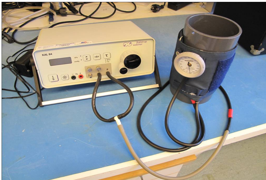
Calibration of blood pressure machine
