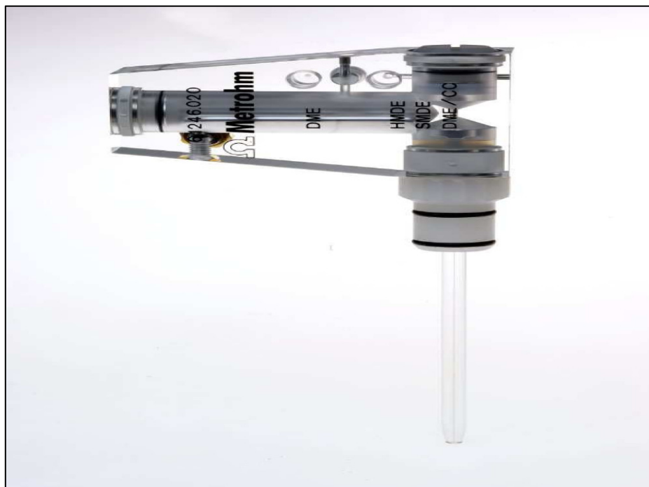
Modern mercury drop electrode
