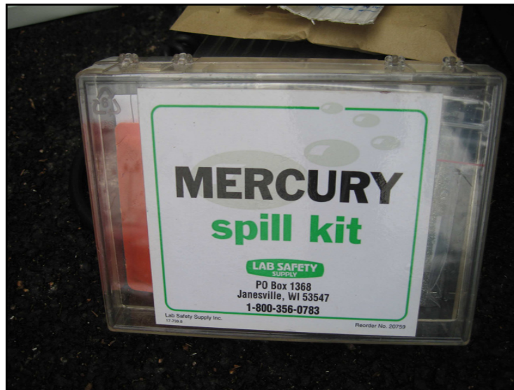
Special Mercury spill kit in case of breakage, leakage
