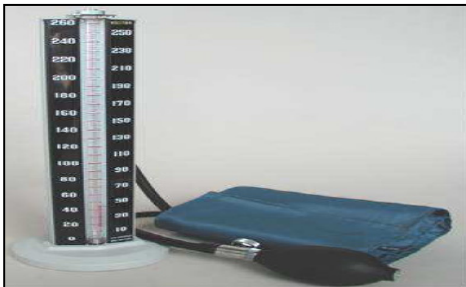
Traditional mercury sphygmomanometer
