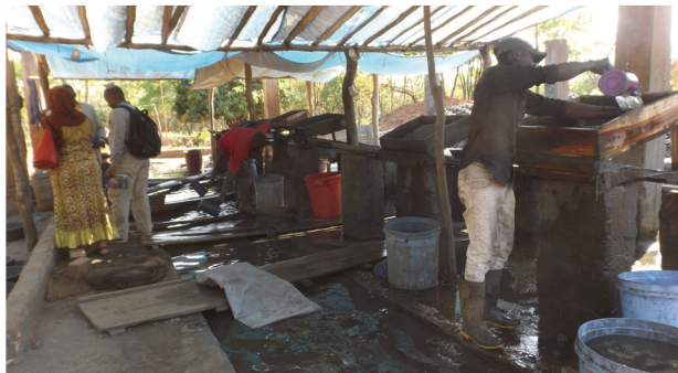
Ore concentrating by sluicing process
